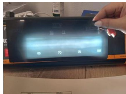
Fig. 5 Radiographic Test Result Evaluation
