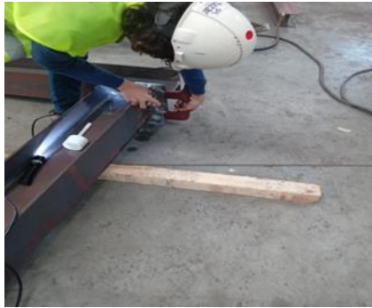
Fig. 3 Magnetic Test Application
