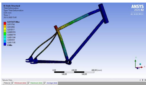
Fig. 5 Total deformation results when 600 N is applied
