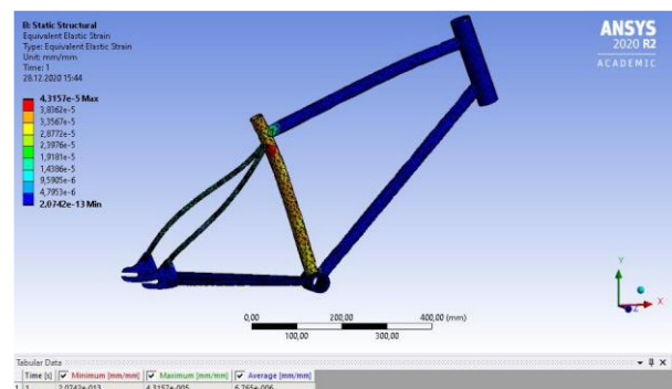
Fig. 7 Equivalent elastic strain results when 600 N is applied
