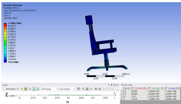
Fig. 21 Equivalent (Von-Mises) Stress of Office Seat
