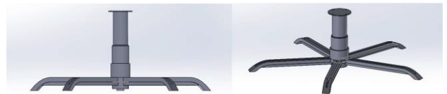
Fig. 18 The Feet Which Supported by 10 mm Thick Feder
