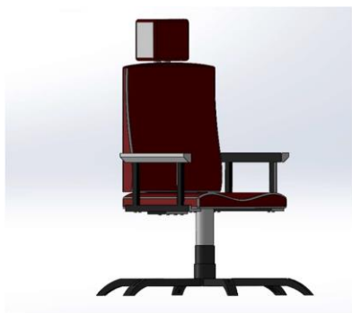
Fig. 4 Side View of Office Seat Made of Aluminum
