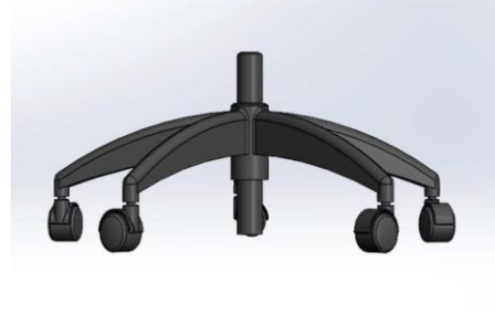
Fig. 11 Office Seat Feet Made of Structural Steel
