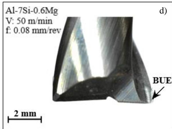
Figure 7. BUL and BUE formation on the cutting edge, a and b)  $V: 110 \text{ m/min}$ ,  $f: 0.08 \text{ mm/rev}$ ; c and d)  $V: 50 \text{ m/min}$ ,  $f: 0.08 \text{ mm/rev}$
