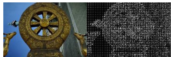
Fig. 4 Obtaining coefficients (right image) by applying DCT to a forged image (left image).
