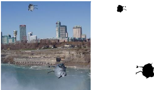
Fig. 2 An image created with copy move forgery method (left) and the mask of the manipulated region of the image (right).
