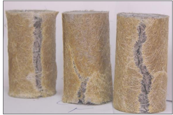
Figure 2. Fracture surfaces of concrete specimens confined by 1-ply FRP.
