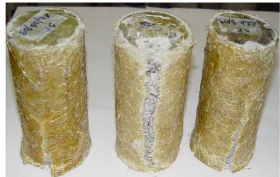
Figure 4. Fracture surfaces of concrete specimens confined by 3-ply FRP.
