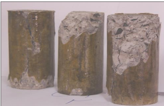
Figure 1. Concrete specimens without reinforcement after crushing.
