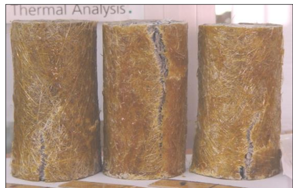
Figure 3. Fracture surfaces of concrete specimens confined by 2-ply FRP.
