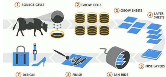
Figure 2. The Process of Lab-Grown Leather ( https://www.tetrafab.com/biofabrication-future-leather/ )
