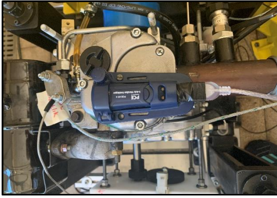
Fig. 4. Connection of the vibration device on the engine
