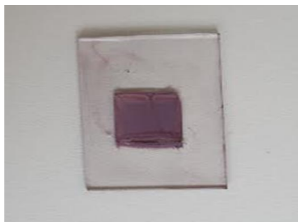
Fig. 3 Working electrode obtained by keeping it in a dye solution prepared with N719 dye
