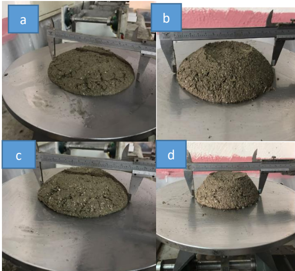
Figure 4. Flow diameter experiment (a) Control (b) 5% UA (c) 10%UA and (d) 20% UA
