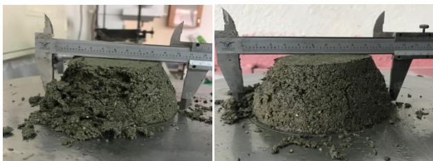
Figure 6 %4 Glass Fiber Spread Test
