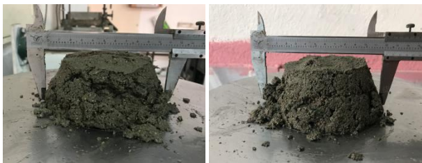
Figure 5 % 2 Glass Fiber Spread Test
