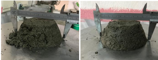
Figure 4 % 1 Glass Fiber Spread Test
