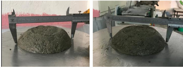
Figure 3 % 0,5 Glass Fiber Spread Test
