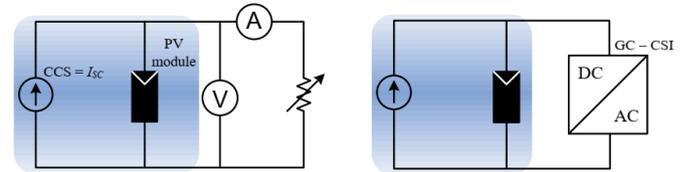
Fig. 4 (a) Test setup for dark I-V,
