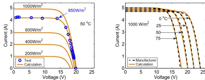
Fig. 3 Non-linear I-V curves for different irradiance and temperature values, for both (a) outdoor tests and (b) values given in the manufacturer's datasheet
