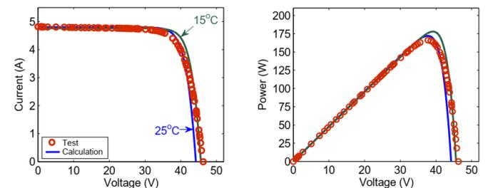
Fig. 5 The nonlinear model shows (a) I-V and (b) P-V curves for temperatures of 15°C and 25°C, as well as dark I-V results at an irradiance of 1000 W/m<sup>2</sup>
