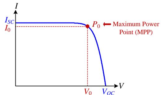
Fig. 1: Typical PV module I-V curve displaying the open-circuit voltage ( $V_{OC}$ ), short-circuit current ( $I_{SC}$ ), maximum power point ( $P_0$ ), voltage at MPP ( $V_0$ ) and current at MPP ( $I_0$ ).
