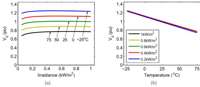
Fig. 2 Variations in voltage with respect to (a) irradiance and (b) temperature at MPP
