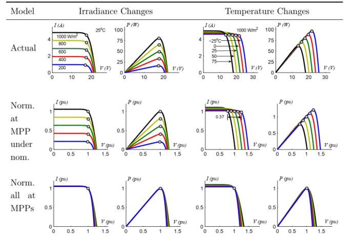
Fig. 2 illustrates the impact of different levels of irradiance and temperature on the maximum power point voltage  $V_0$  of a photovoltaic (PV) module. Fig. 2(a) depicts the irradiance effect. The voltage  $V_0$  experiences a significant decrease with an increase in temperature, as illustrated in Fig. 2(b). This is attributed to the fact that the voltage remains mostly constant, except for low levels of irradiance.
