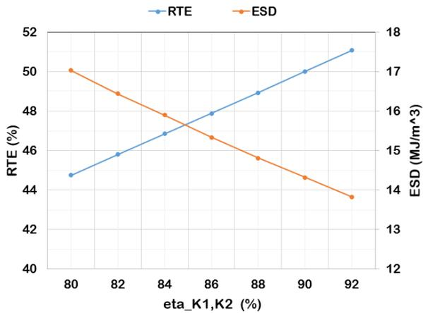
**Figure 4.** Influence of isentropic efficiency of compressors on  $\eta_{RTE}$  and ESD.
