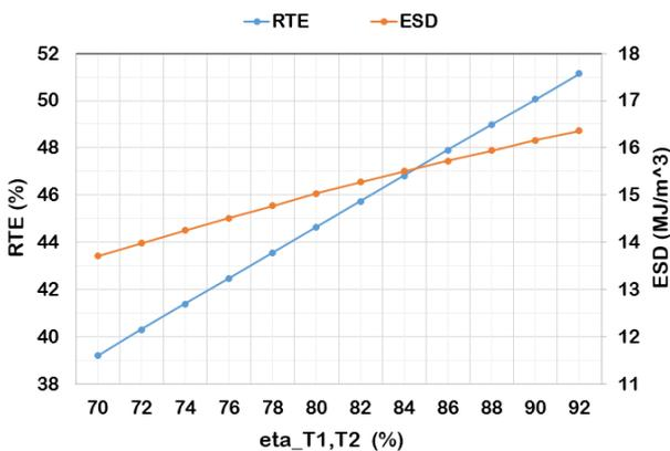
**Figure 5.** Influence of isentropic efficiency of turbines on  $\eta_{RTE}$  and ESD.
