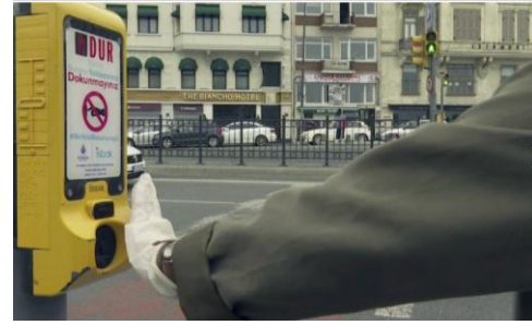
Fig. 2 Contactless pedestrian signal [2].
