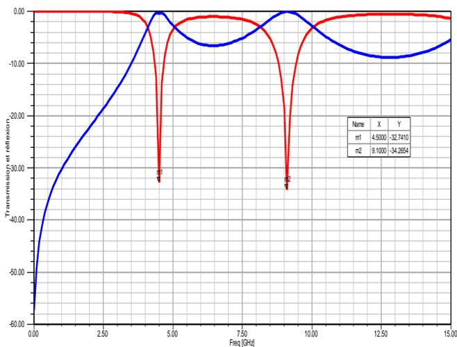
Fig. 7 Transmission and reflection of the proposed DBBPF.
