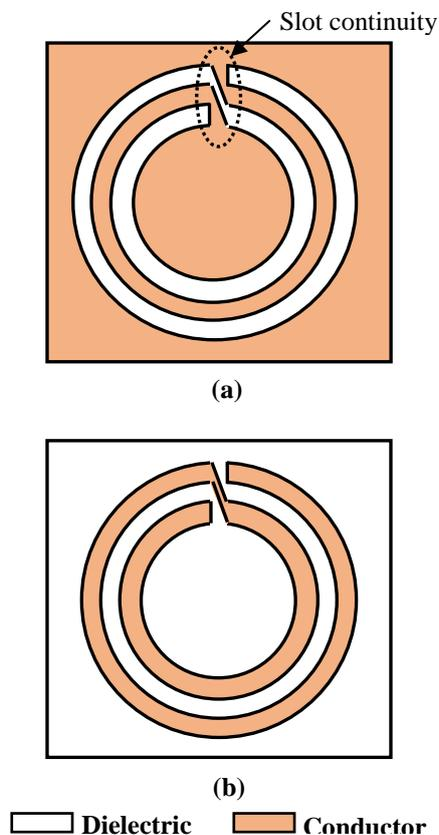
Fig. 1 Comparison between (a) CSRR, (b) SRR circular spiral shape
