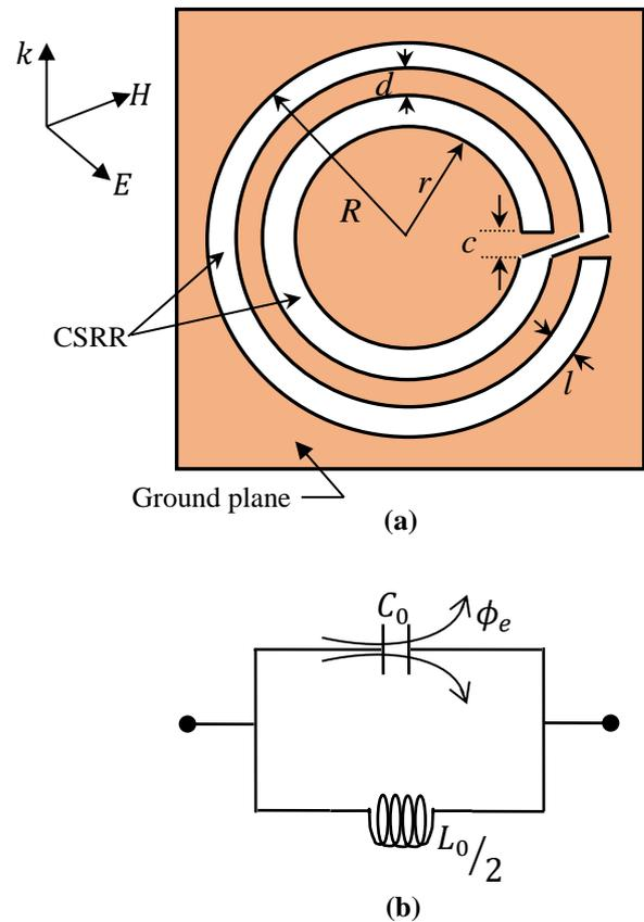
Fig. 2 Presentation of CSRR (a) Polarization, (b) equivalent electrical circuit
