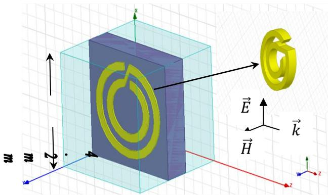
Fig. 3 Polarization of the SRR along  $OX$ .
