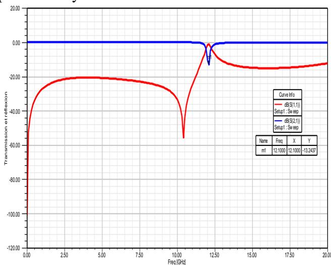
Fig. 4 Transmission and reflection SRR
