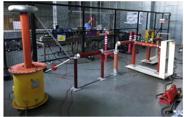
Fig. 3 Impulse voltage generator in laboratory
