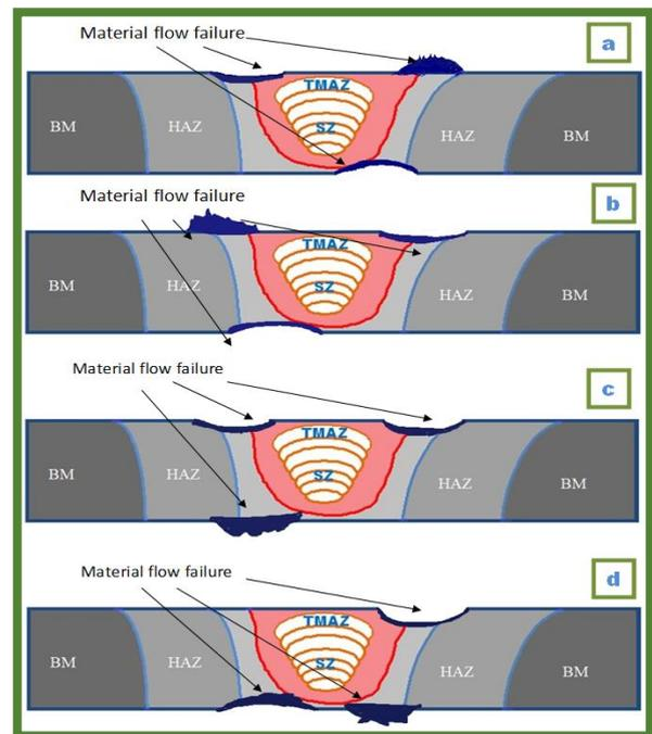
Fig. 3 Material flow errors caused by the rotation direction of the tool; a) Tool rotation clockwise with right-helix pin, b) Tool rotation counterclockwise with right-helix pin, c) Tool rotation clockwise with left-helix pin, d) Tool rotation counterclockwise with left-helix pin
