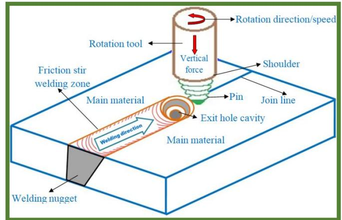
Fig. 1 Schematic of the FSW technique
