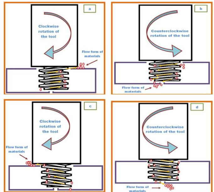
Fig. 2 Material transport based on tool rotation direction and pin helix configuration; a) Tool rotation clockwise with right-helix pin, b) Tool rotation counterclockwise with right-helix pin, c) Tool rotation clockwise with left-helix pin, d) Tool rotation counterclockwise with left-helix pin
