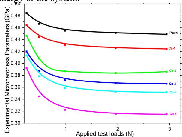
Figure 1. Differentiation of microindentation test load hardness parameters
