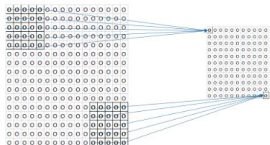
Figure 2.1 Extraction of Feature Maps with the Convolutional Layer [15]
