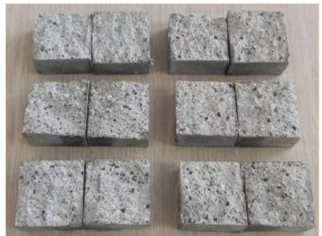
Figure 6. General view of the specimen after splitting tensile test
