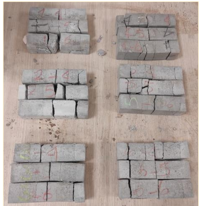
Figure 5. General view of the specimen after compression test
