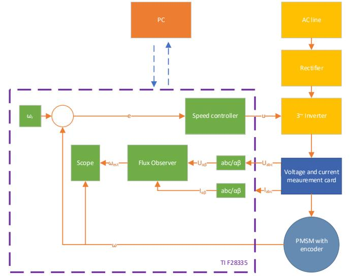
Fig. 1 Block diagram of PMSM system
