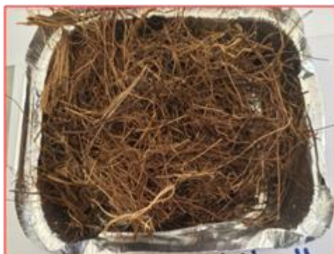
Fig 4. Treatment with hot water at 80°C + 0.5% NaOH.
