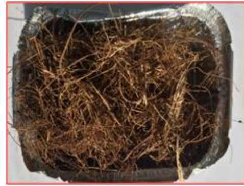
Fig 5: Treatment with hot water at 80°C + 1% NaOH.
