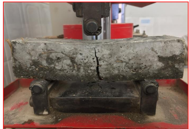
Fig 6. Prismatic test tubes 4x4x16 cm 3 .
