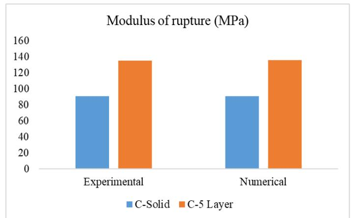
Fig. 2. Results of modulus of rupture
