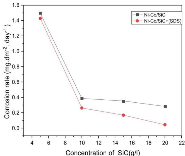
Fig. 2 depicts the variation of the corrosion rate as a function of SiC concentration, along with the influence of sodium dodecyl sulfate (SDS) [1].
