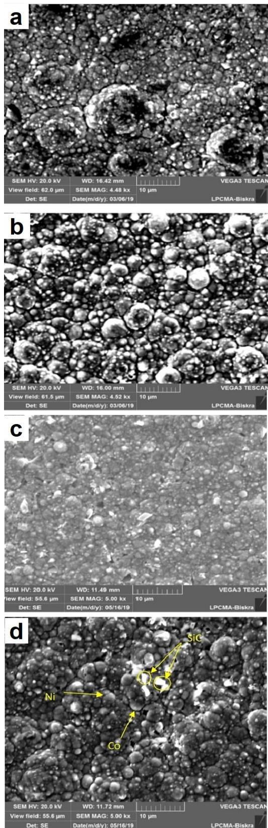
Fig. 1. SEM images of : Ni-Co/SiC coatings at: (a) 5 g l<sup>-1</sup>, (b) 10 g l<sup>-1</sup>. SEM images of Ni-Co/SiC with organic additive (SDS) coatings at: (c) 5 g l<sup>-1</sup>, (d) 10 g l<sup>-1</sup> [1].
