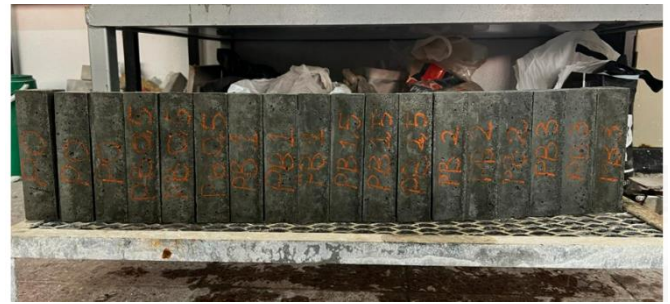
Figure 2. Basalt fiber reinforced raw perlite aggregate cement mortar samples
