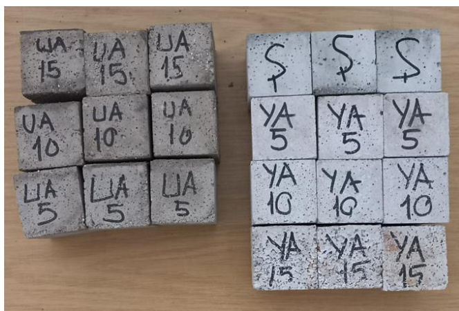
Figure 1. Samples of AAC mortar with Additive Aluminum Chip
