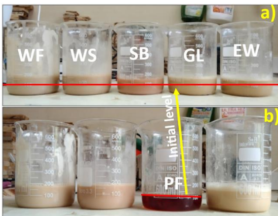
Fig. 1 Foamed PF samples (a), and initial level (b)
