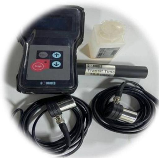
Figure 4: UPV device used in the present study
