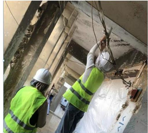
Figure 3: Collecting RH values of beams and columns
