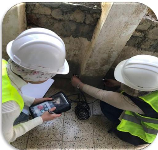
Figure 5: Collecting UPV values on beams and columns
