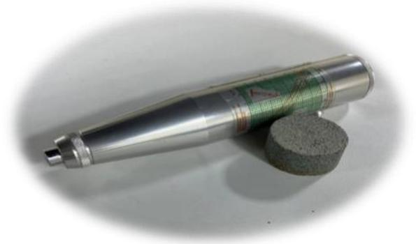
Figure 2: RH device used in the present study
