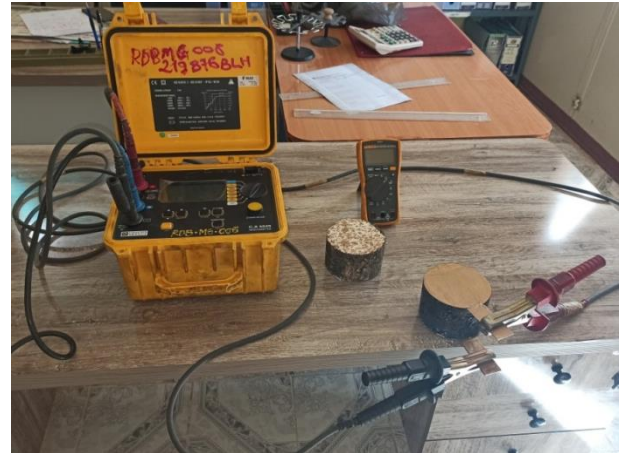
Fig. 4. Electrical resistivity test
