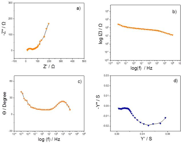
Fig. 4 EIS plots of rGO/CuO/PPy nanocomposite a) Nyquist plot, b) Bode-magnitude plot, c) Bode-phase plot, d) Admittance plot.
