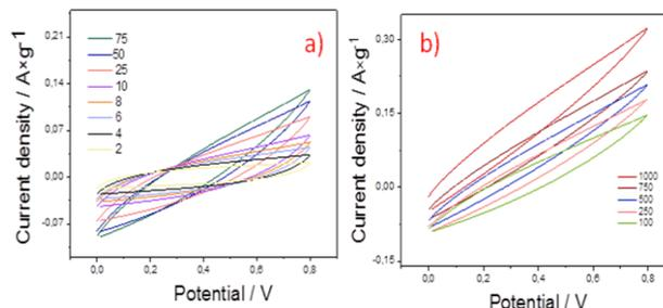
Fig. 1 C V plots of rGO/CuO/PPy nanocomposite at different scan rates, a)  $1000\text{-}100 \text{ mV}\times\text{s}^{-1}$ , b)  $75\text{-}2 \text{ mV}\times\text{s}^{-1}$ .
