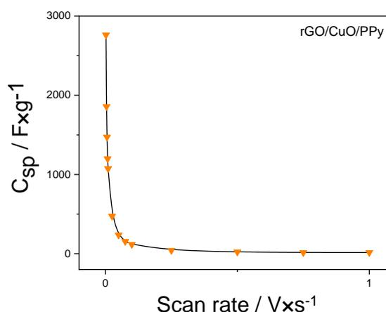
Fig. 2  $C_{\text{sp}}$  vs. Scan rate plot of rGO/CuO/PPy nanocomposite at different scan rates from  $1000$  to  $2 \text{ mV}\times\text{s}^{-1}$ .
