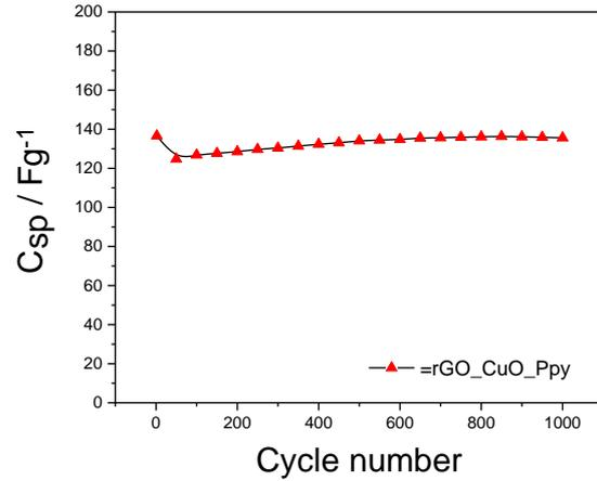
Fig. 5 Stability tests of rGO/CuO/PPy nanocomposite at a scan rate of  $100 \text{ mV} \times \text{s}^{-1}$ , 1000 charge-discharge measurements.
