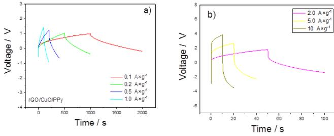
Fig. 3 GCD plots of rGO/CuO/PPy nanocomposite at constant current density from  $0.1 \text{ A} \times \text{g}^{-1}$  to  $10 \text{ A} \times \text{g}^{-1}$ .
