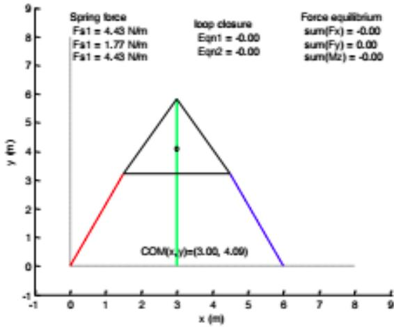
Fig. 3. Second equilibrium position of 3-DOF mechanism
