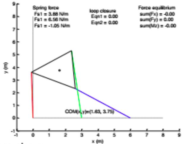
Fig. 2. First equilibrium position of 3-DOF mechanism
