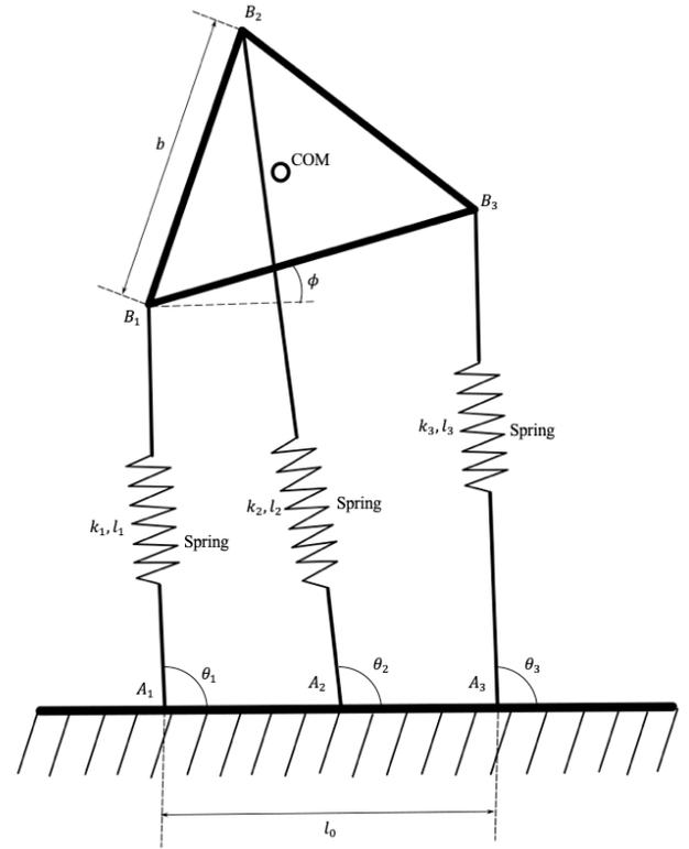
Fig. 1. The planar 3 degree-of-freedom parallel mechanism
