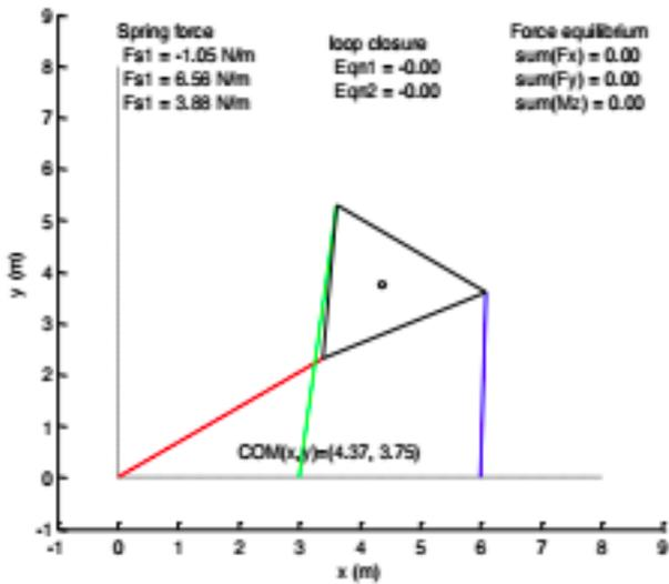
Fig. 4. Third equilibrium position of 3-DOF mechanism
