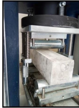
Fig. 6. Static diagram and device of the tensile test by bending.
