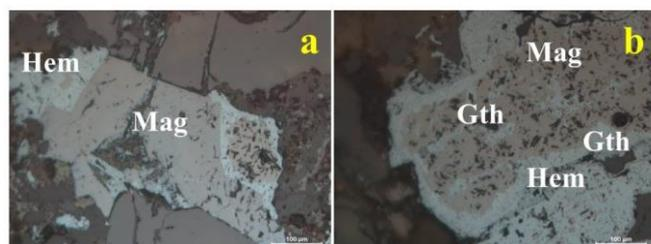
Fig. 4 Ore microscopy views of ore samples collected from the skarn mineralization. Abbreviations: (Mag) magnetite, (hem) hematite, (Gth) Goethite
