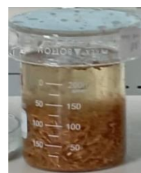
Figure 5: Impregnation process in H_3PO_4 and 0.5 gm of AlCl_3 for 24 hr
