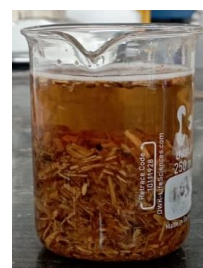
Figure 4: Acetone and distilled water impregnation for 24 hours.
