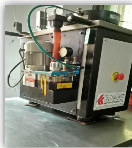
Fig. 1 Koehler k93500 Pin on disc tribo-tester
