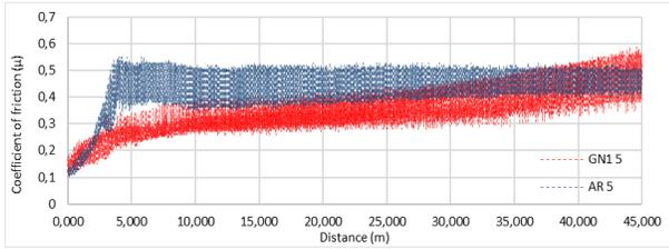
Fig. 6 Friction coefficient changes of AR and GN1 specimens at 5 mm/s sliding speed
