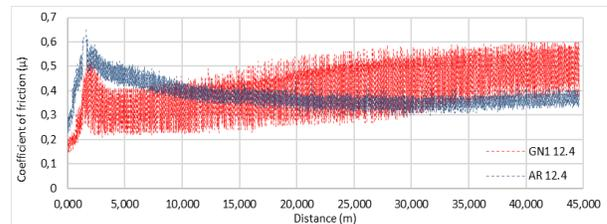
Fig. 5 Friction coefficient changes of AR and GN1 specimens at 12.4 mm/s sliding speed
