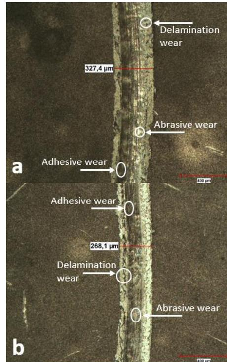
Fig. 10 Optical microscope images of the wear groove and track width for GN2 specimen: (a) 12.4 mm/s, (b) 5 mm/s
