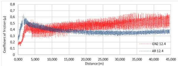
Fig. 7 Friction coefficient changes of AR and GN2 specimens at 12.4 mm/s sliding speed
