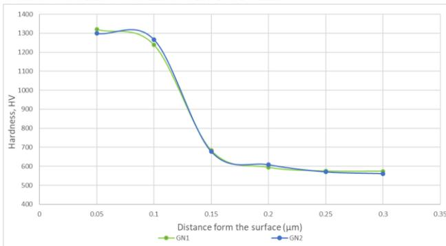
Fig. 5 Hardness distribution of plasma- and gas-nitrided DIN 1.2367 steel specimens
