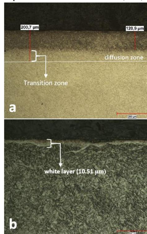
Fig. 3 Optical microscope images of the gas-nitrided specimen GN2 at 500 °C for 12 h ( $Kn:18$ )
