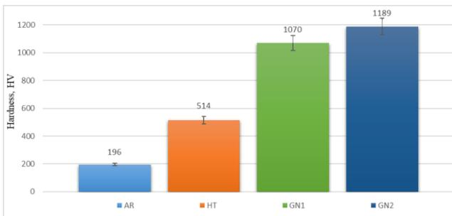
Fig. 4 Hardness results of the test specimens
