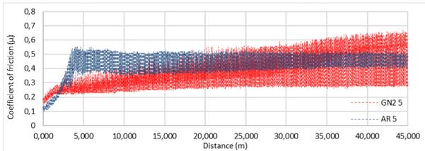
Fig. 8 Friction coefficient changes of AR and GN2 specimens at 5 mm/s sliding speed
