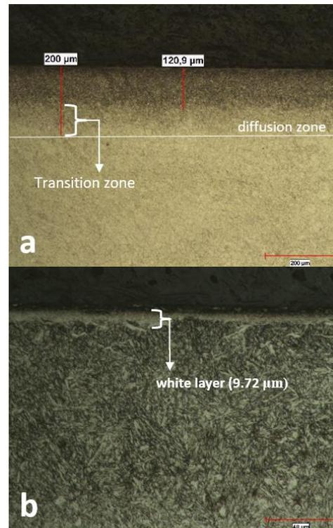
Fig. 2 Optical microscope images of the gas-nitrided specimen GN1 at 500 °C for 12 h ( $Kn:4$ )
