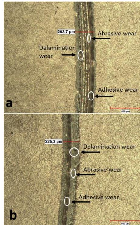
Fig. 9 Optical microscope images of the wear groove and track width for GN1 specimen: (a) 12.4 mm/s, (b) 5 mm/s
