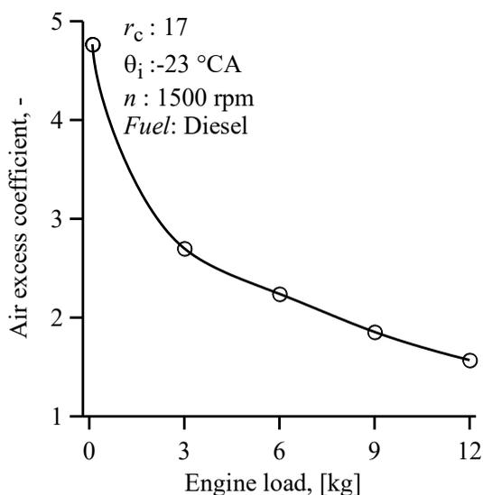
**Fig. 3.** Variation of air excess coefficient with engine load
