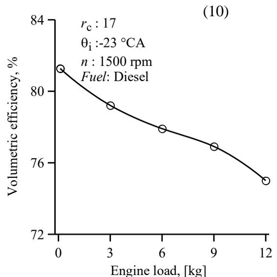
**Fig. 2.** Variation of volumetric efficiency with engine load
