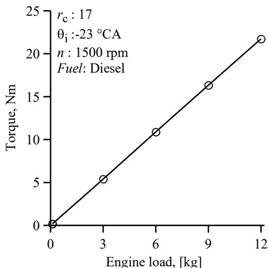
**Fig. 4.** Variation of torque with engine load
