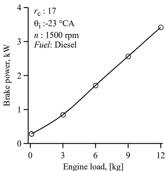
**Fig. 5.** Variation of brake power with engine load
