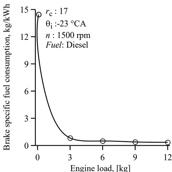
**Fig. 6.** Variation of brake specific fuel consumption with engine load
