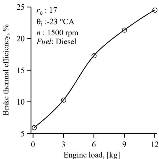
**Fig. 7.** Variation of brake thermal efficiency with engine load
