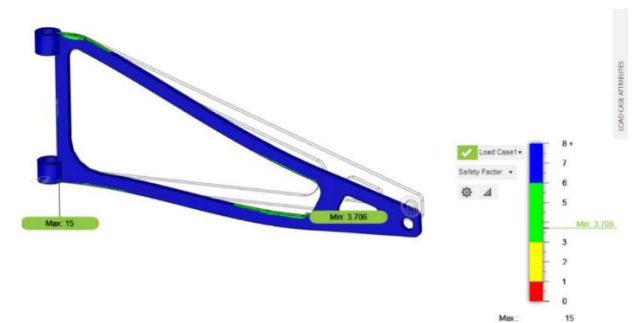
Fig 12. Security Factor of Topology Optimized Model
