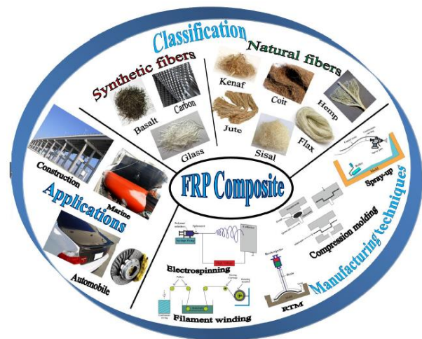
Figure 1. Classification, production techniques, and applications of fiber reinforced composites [24].
