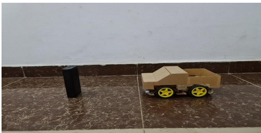
Fig.8: Vehicle detects obstacle within 55cm
