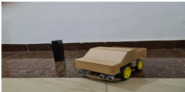
Fig.10: Detections no obstacle continues and again moves on a forward path
