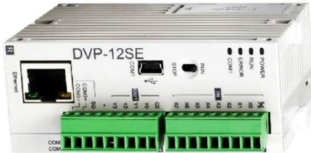
Fig. 1 Delta DVP-12SE brand PLC
