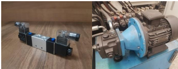
Fig. 2 Example of solenoid valve and motor controlled by PLC device
