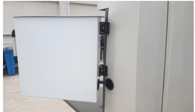
Fig. 15 Connection of the test panel
