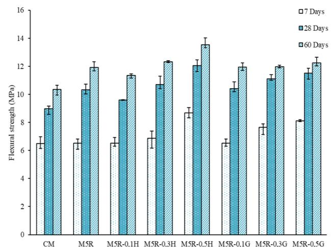
Fig.3. Flexural strength of differently prepared mortars.
