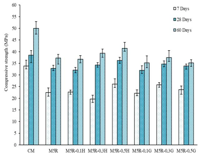
Fig 4. Compressive strength of the various prepared mortars.
