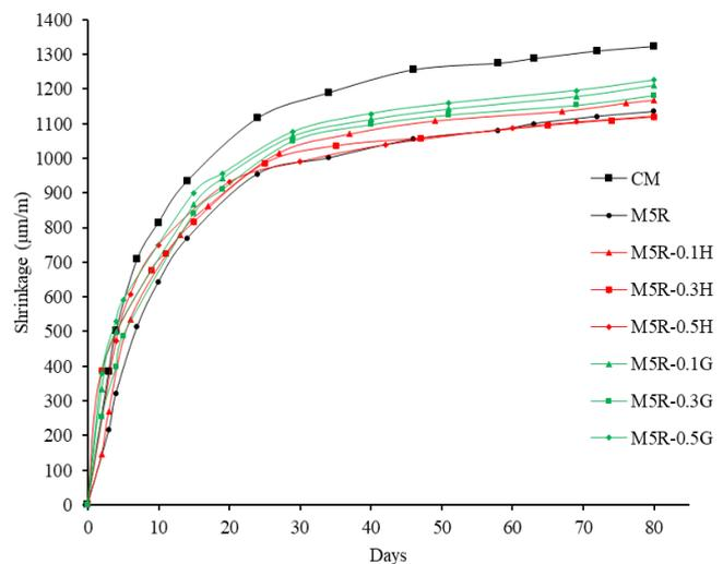
Fig.5. Total Shrinkage of the different mixtures.
