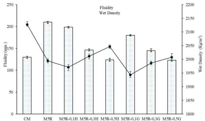
Fig2. Fluidity and wet density of different mixtures.
