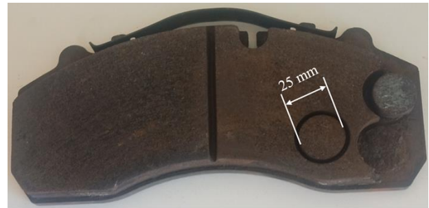
Fig. 1 Commercial vehicle disc brake pad and sampling images
