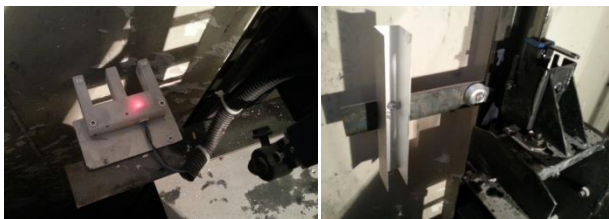
Fig. 11 Sensor and "U" shaped barrier after installation
