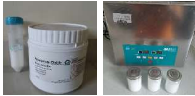
Fig. 6 SDS surfactant, Al 2 O 3 nanofluid and ultrasonic bath device
