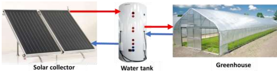
Figure 2. Solar greenhouse heating system
