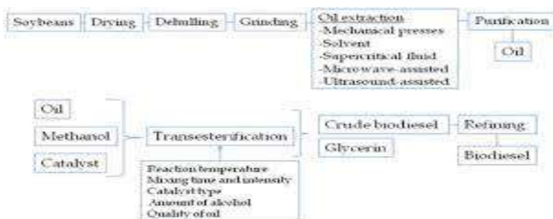
Fig.2 The process of extracting oil from soybeans to produce biodiesel (11). Chemical Extraction :
