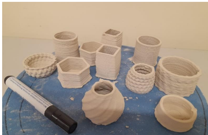
Figure 6. The printed models with the clay of 30% water content.
