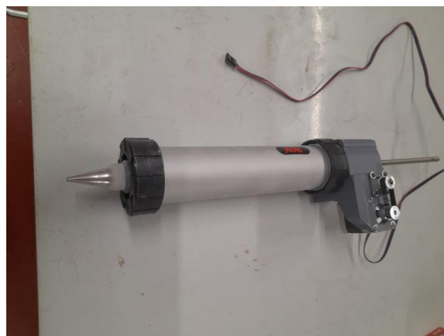
Figure 5. The realized direct clay extruding system.
