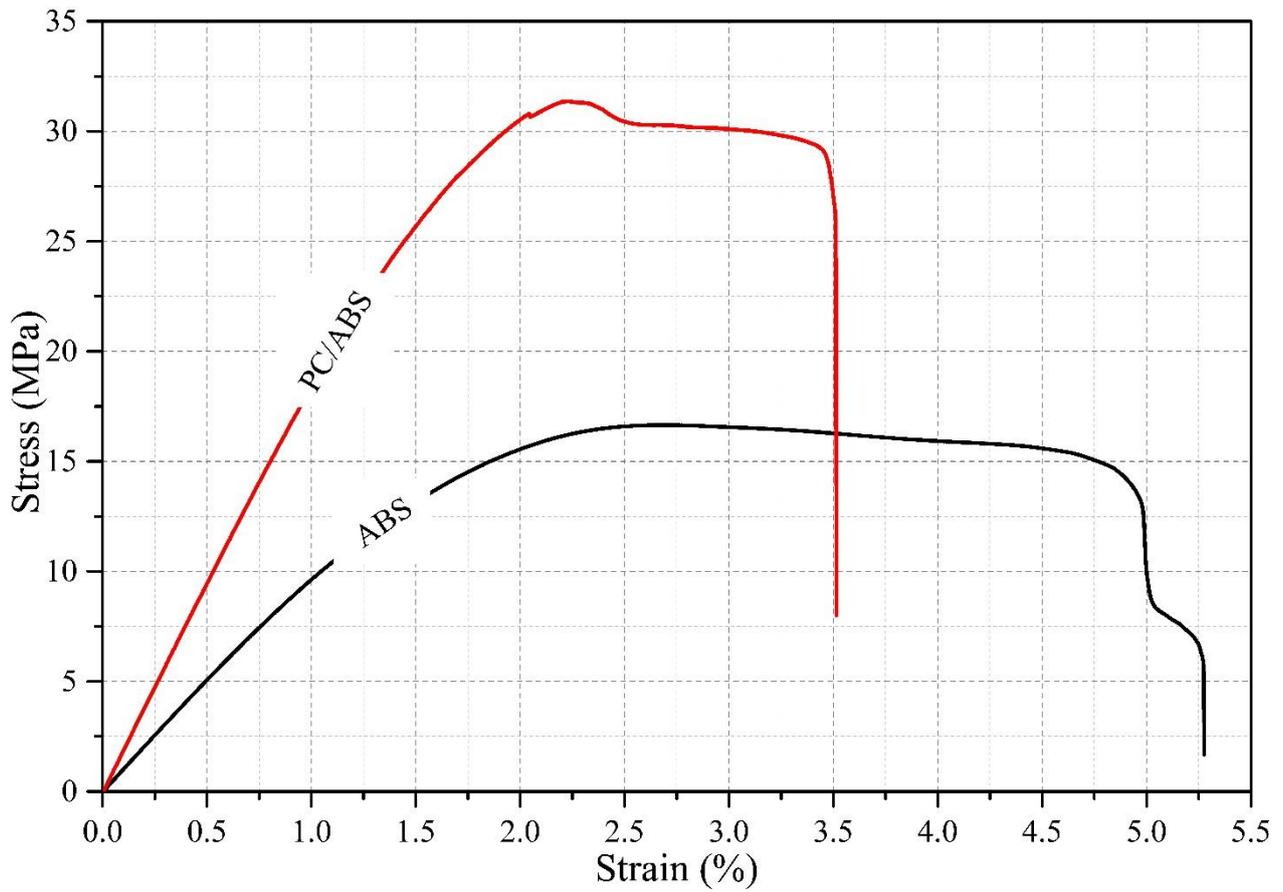
Figure 2. 3D printed materials' representative curves for uniaxial tensile test behaviors
