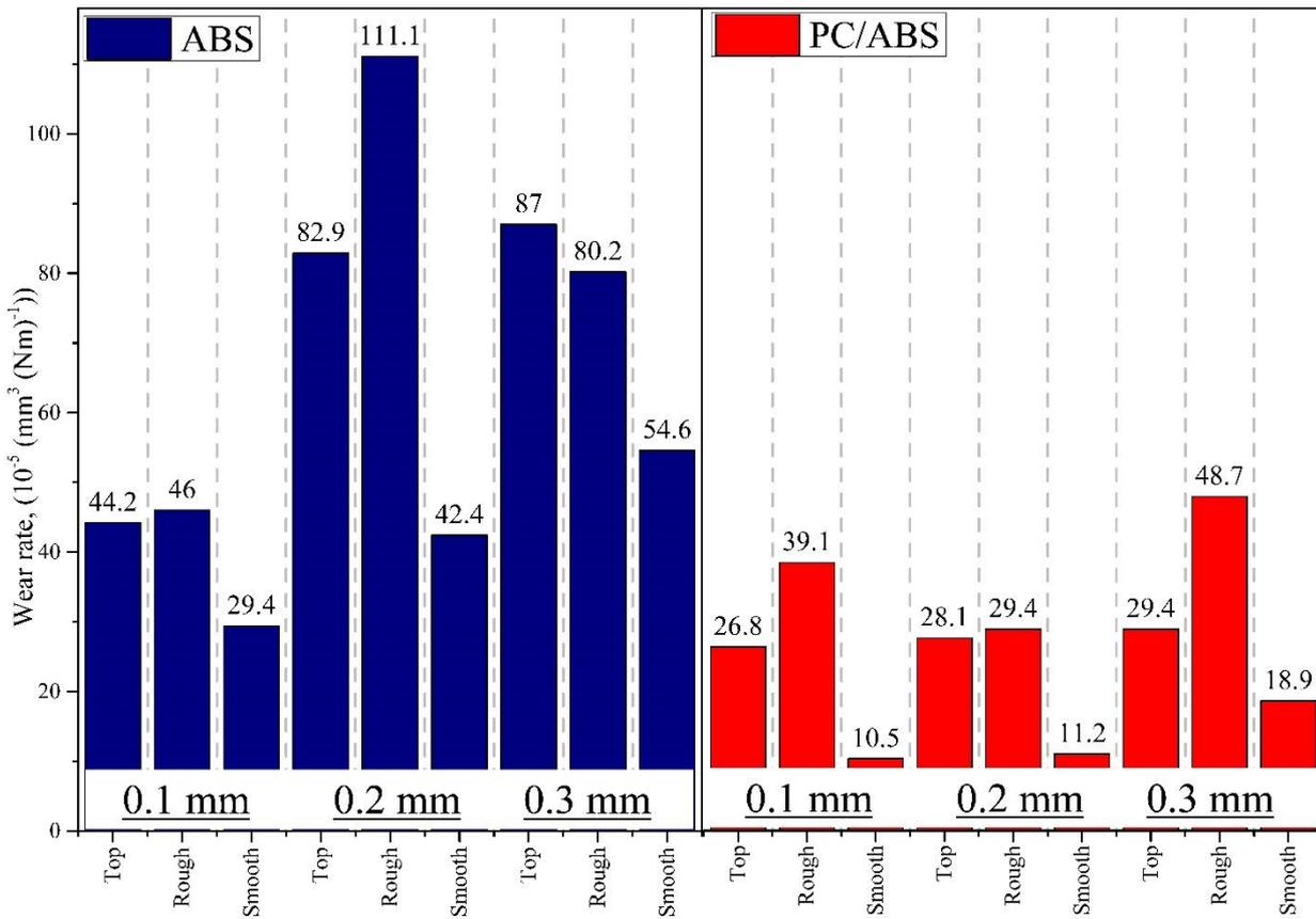
Figure 3. A comparative graph depicting wear rates for various surface types and layer thicknesses
