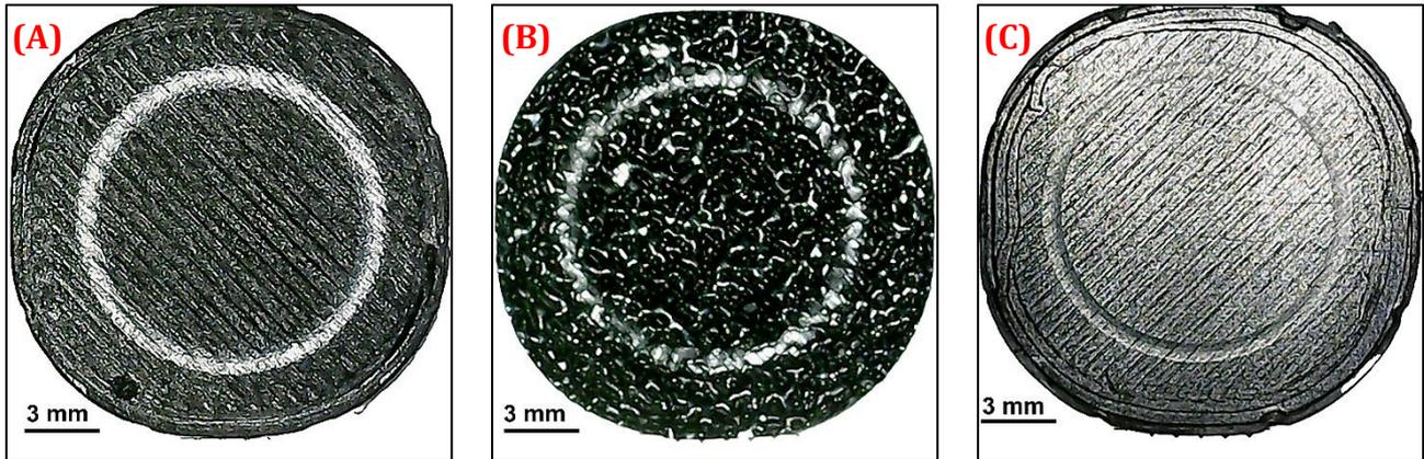
Figure 1. Optical microscope images of samples with different surface patterns; a) Top surface, b) Bottom surface rough, c) Bottom surface smooth
