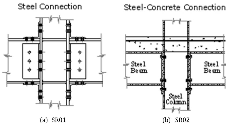
Fig 4: conception of the semi-rigid joints (a) and (b)
