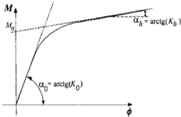
Fig 3: moment rotation behavior of semi rigid joint (M-φ).
