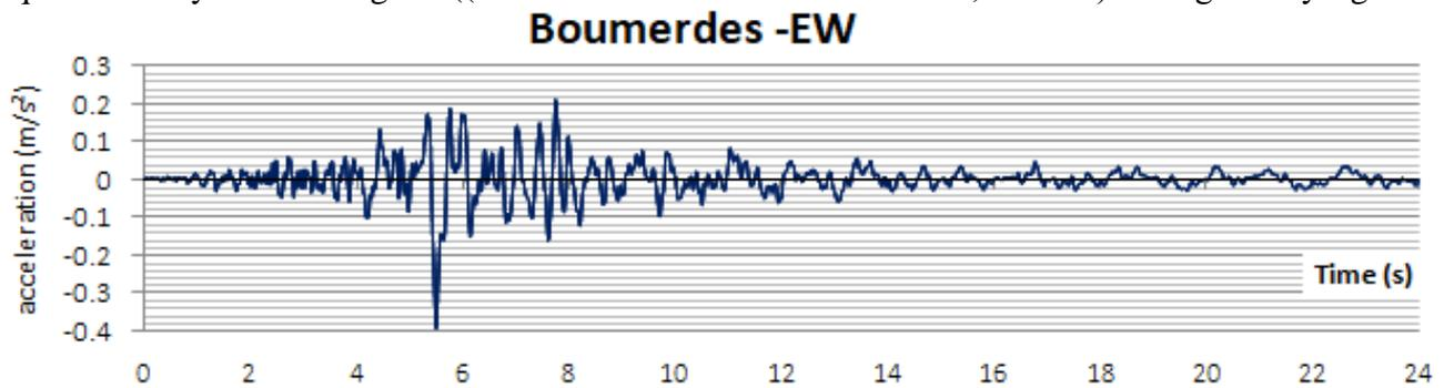
Fig 6: Recording of the Boumerdès earthquake in the EW direction with a  $PGA= 0.394 m/s^2$ .
