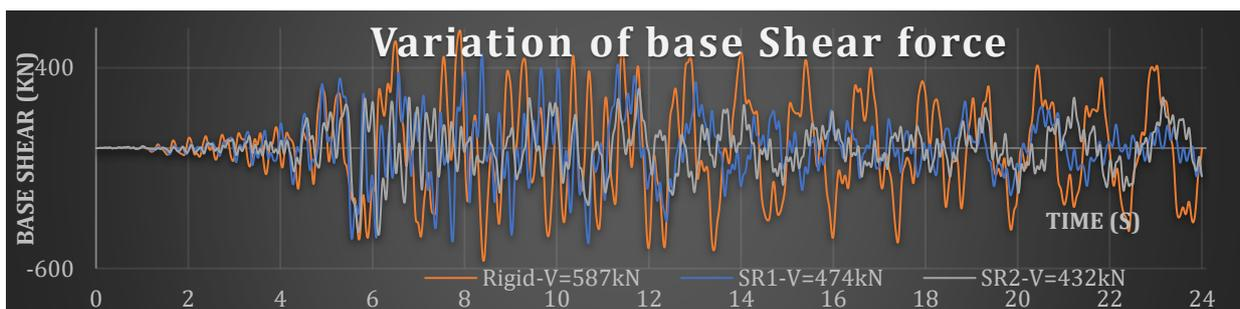
Fig 9: Seismic base Shear force variation
