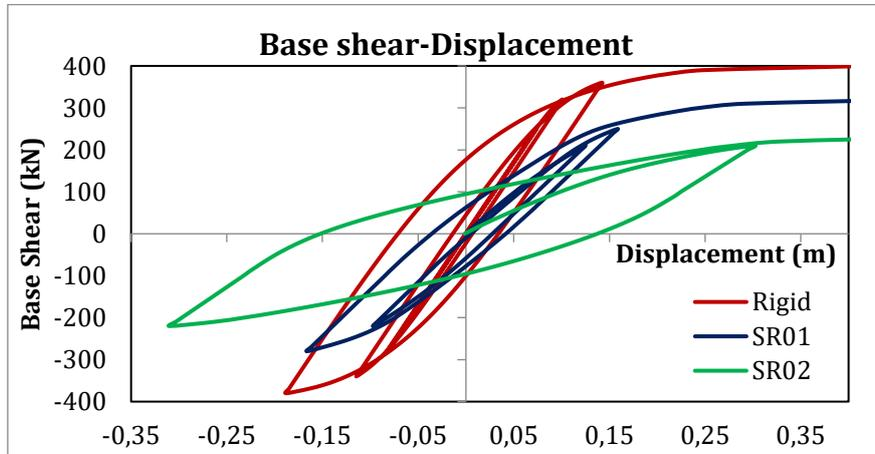
Fig10: The hysteresis loops obtained through cyclic analysis of the structure.
