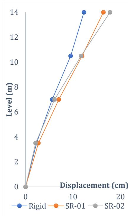
Fig 8. Maximum displacement of each story
